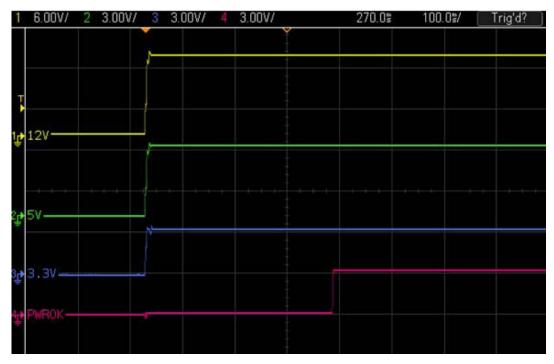
The module will remain in power-off state as long as the PWR\_OK is driven by carrier board hardware. The conga-TC675r supports the controlling of ATX-style power supplies. If you do not use an ATX power supply, do not connect the conga-TC675r pins SUS\_S3, 5V\_SB, and PWRBTN#.
